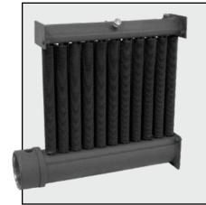
The *ExCaliber*<sup>™</sup> vacuum sealed liquid-to-air heat exchanger core is constructed using rugged, copper-free, roll-formed aluminum fins and protected by a pressure relief device. automatic reset high limit, and a back-up manual reset high limit.
